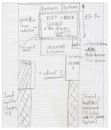
Figure 3. The first sketch of a top view of the internal space
