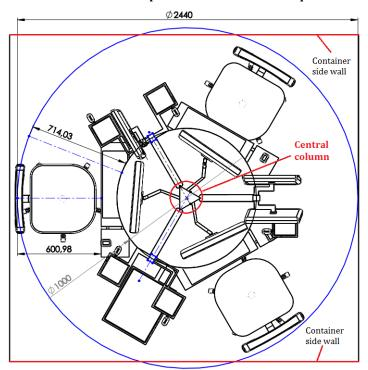
Figure 9. Ground wireframe view of the operators' workstation complex
